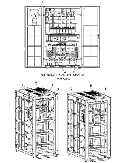
Figure 40 Liebert<sup>®</sup> NX<sup>™</sup> 160-200kVA UPS to 49" battery cabinet interconnection
